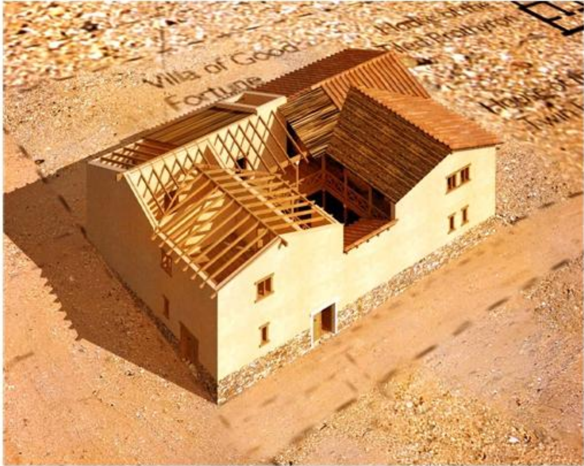
Villa of Good Fortune in ancient Olynthos. The roofs of the upper floor were made of wood and had tiles of clay.
