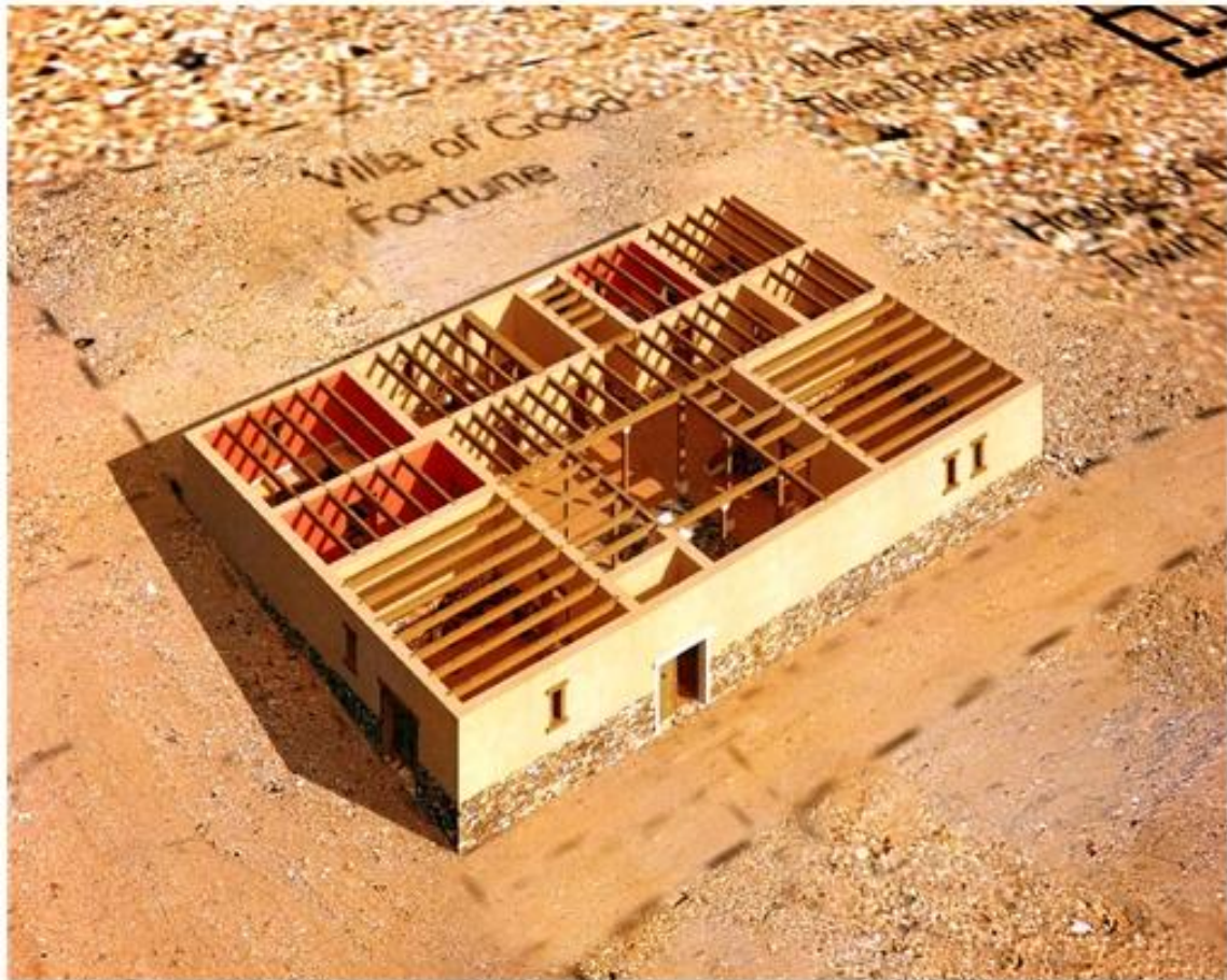
Villa of Good Fortune in ancient Olynthos. The wooden beams supporting the first floor. Wood, together with raw earth, was the most bioclimatic among the main construction materials available in ancient times.
