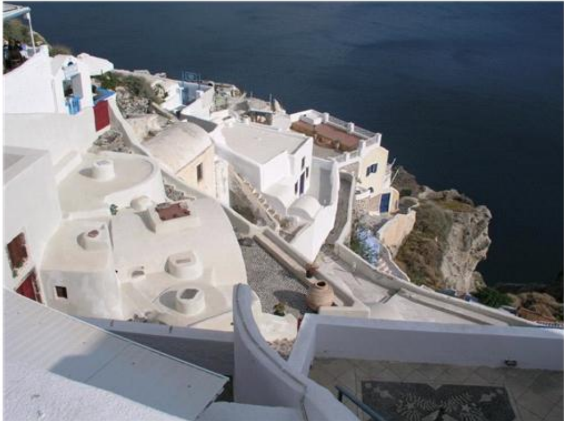
Islands of Santorini (above) and Patmos (below). The roofs have insulation made of earth and seaweeds and they are flat, in order to collect the rain water.
