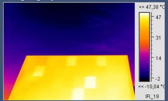
IR thermography of a new 50W<sub>p</sub> sc-Si PV module. Two hot cells exhibit temperature higher by about 6°C from the average temperature of the module.
